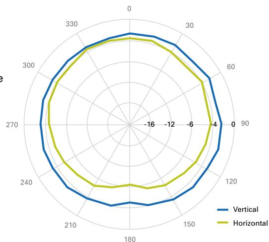
\*Readtenna<sup>TM</sup> 900 has excellent azimuthal pattern and average gain of -2dB relative to a dipole. Note that an ideal circularly polarized antenna is -3dB relative to a dipole.
